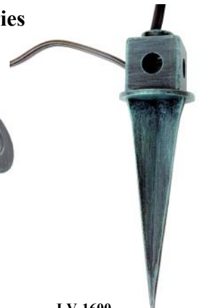
LV-1600 Cast Aluminum Spike Ht.: 10" Includes 6" 14/2 Cable Pipe Thread: ½"
